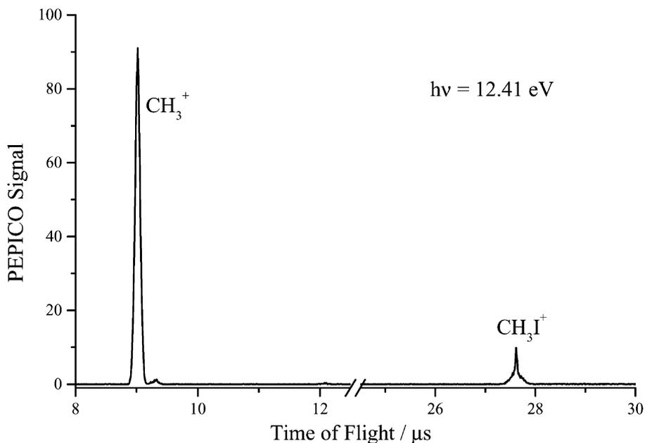
Fig. 4. The photoelectron photoion coincidence mass spectrum of  $\text{CH}_3\text{I}$  in the vicinity of the dissociative ionization onset. The small peak to the right of the  $\text{CH}_3^+$  peak at  $9\ \mu\text{s}$  is due to the  $^{13}\text{C}$  isotope. The two-component shape of the parent ion peak at  $17.6\ \mu\text{s}$  is a result of the effusive jet that gives rise to the sharp peak on top of the thermal background peak.
